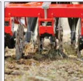
Individually sprung disc openers with easy change discs, seals and bearings are available as an option
