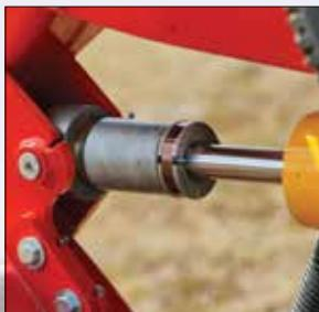
Easy to set depth adjustment with a collar and threaded shaft adjuster
