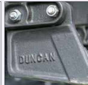
Duncan 'T' boots have extra strength with Ni-hard steel and a tungsten tile on the leading edge
