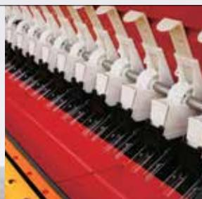
25mm coil tines for superior strength and consistent seeding
